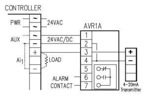
The AVR1A is powered from the controllers AUX power output. *Power supply note: AVR1A's terminal 2 is common to the input, and the AUX is common to the controllers.* The 4-20mA signal is fed into the AVR1A where a 249  $\Omega$  ½ watt resistor provides the load to produce a 1-5VDC signal which both the AVR1A and the controller uses. If the jumper on the AVR1A is left open and external 249  $\Omega$  load resistor should then be connected across the controllers input to (-) common.
