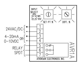
The AVR1A uses a half-wave bridge rectifier, term #2 of AC line is connected to input common term #4. If your output common is not common to one side of the 24VAC line then an isolation transformer is *RECOMMENDED* to avoid ground loop problems.
