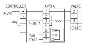
The AVR1A is powered from the same 24VAC as the controller. (Power supply note: Both the AVR1A's input common (-) and the controller's output common (-) share one side of the 24VAC line). The 4-20mA signal is fed into the AVR1A's input and out to the valve's input as a three wire connection. If the valves input impedance is less than 250V then an additional load resistor is added between to AVR1A and the valve. This provides a total voltage drop of 1-5VDC to drive the AVR1A's input.
