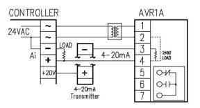
The AVR1A is powered from an isolation transformer so that the input commons (-) of both devices, are isolated from each other. This allows the inputs of two devices to be connected in series, otherwise the second input in the loop would be shorted.
