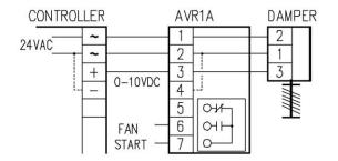
The AVR1A is powered from the same 24VAC as the controller. (Power supply note: Both the AVR1A's input common (-) and the Controller's output common (-) share one side of the 24VAC line). The 0-10VDC signal is fed into the AVR1A's input and out to the damper motor's input as a three wire connection.
